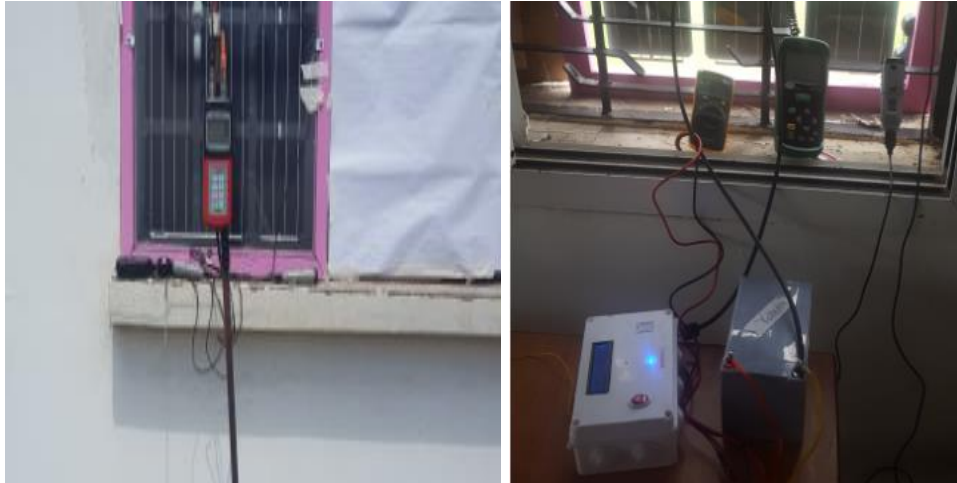
Figure 18: Arrangement and measurements of the temperatures and humidity.
