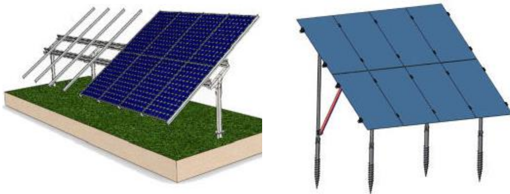
Figure 4: ORPV installation: Photovoltaic system in open rack installation configuration (Kumar, Reddy & Praveen, 2017).
