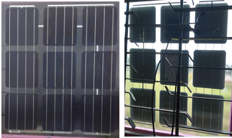
Figure 16: Side view of in and out of the semi-transparent PV window glazing.
