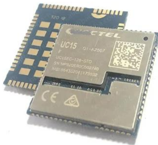
Figure 27: The UC15-3G module (Empowerlaptop, 2022)
