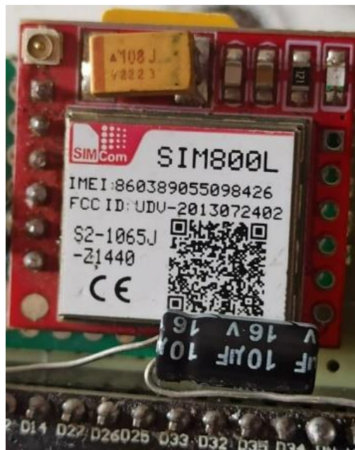
Figure 28: The SIM800L GSM Module
