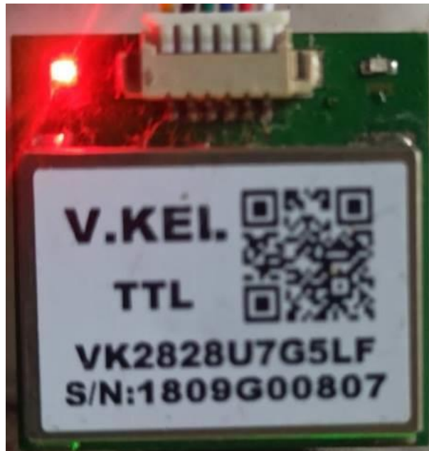
Figure 26: The V.KEI GPS Module
