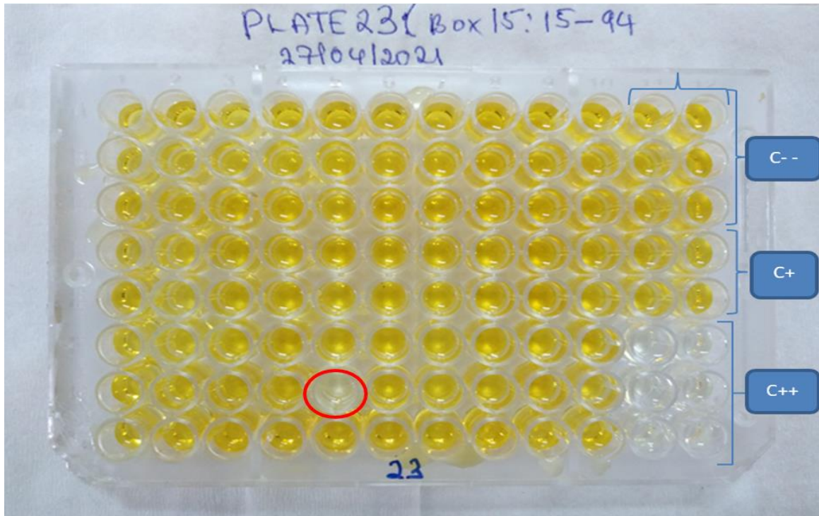
Figure 5: Prepared ELISA plate after the addition of OPD and incubation ready to be set in a microplate reader spectrophotometer
