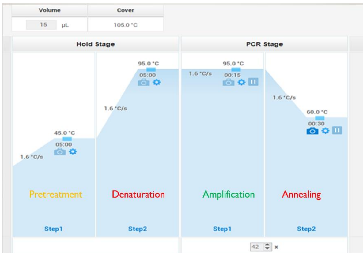
Figure 17: The PCR steps and conditions (Temperature and Time) for the B. abortus and B. melitensis detection
