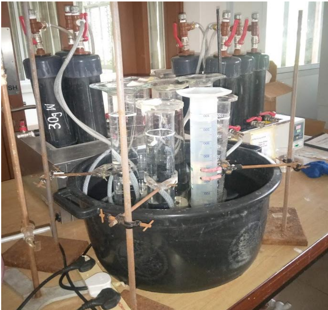
Plate 2: A photograph depicting a laboratory-scale experimental setup designed to optimize zero-valent iron (ZVI) dosages in anaerobic digestion
