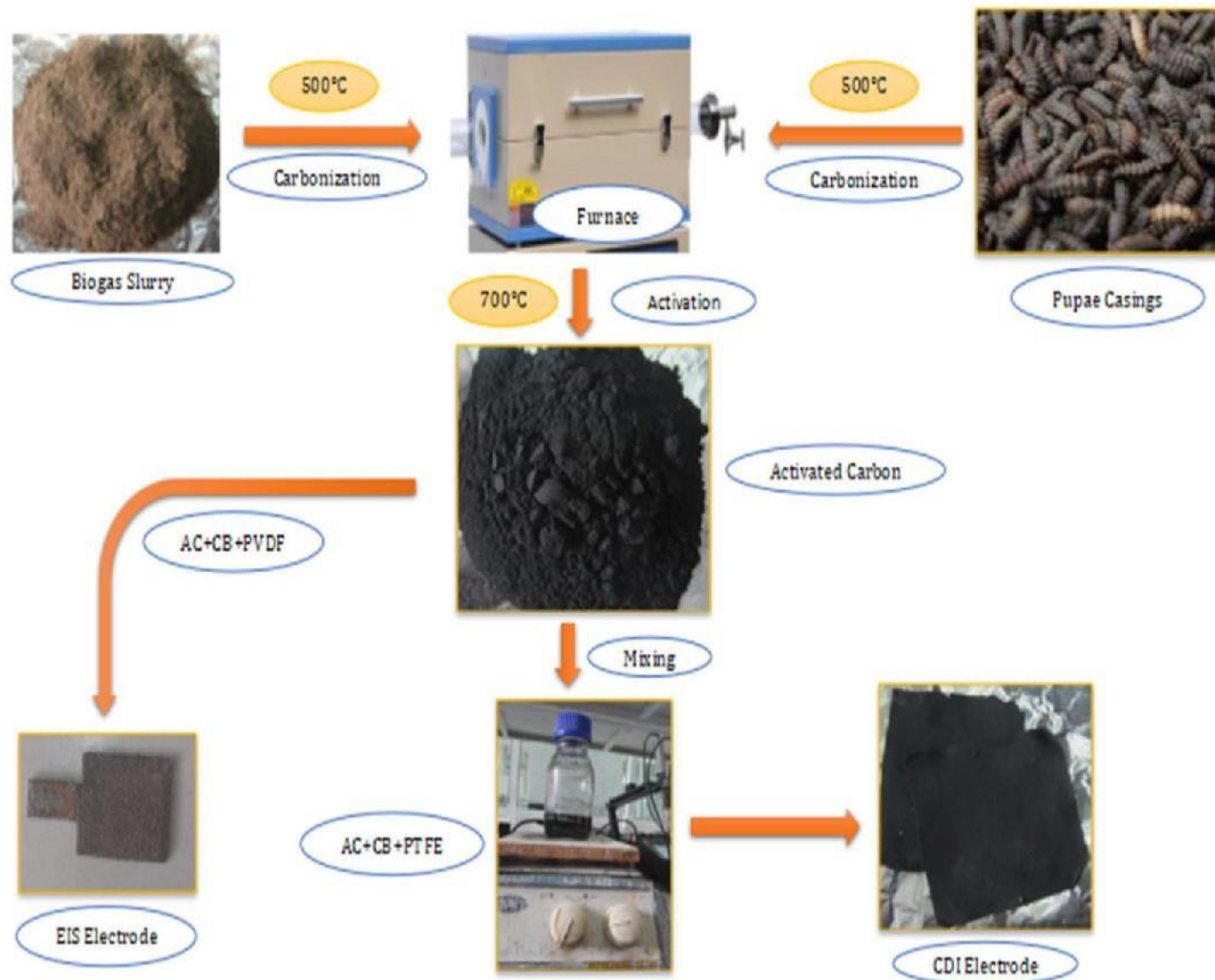
Figure 3: Schematic description of the synthesis of carbon from biogas slurry and pupae casings
