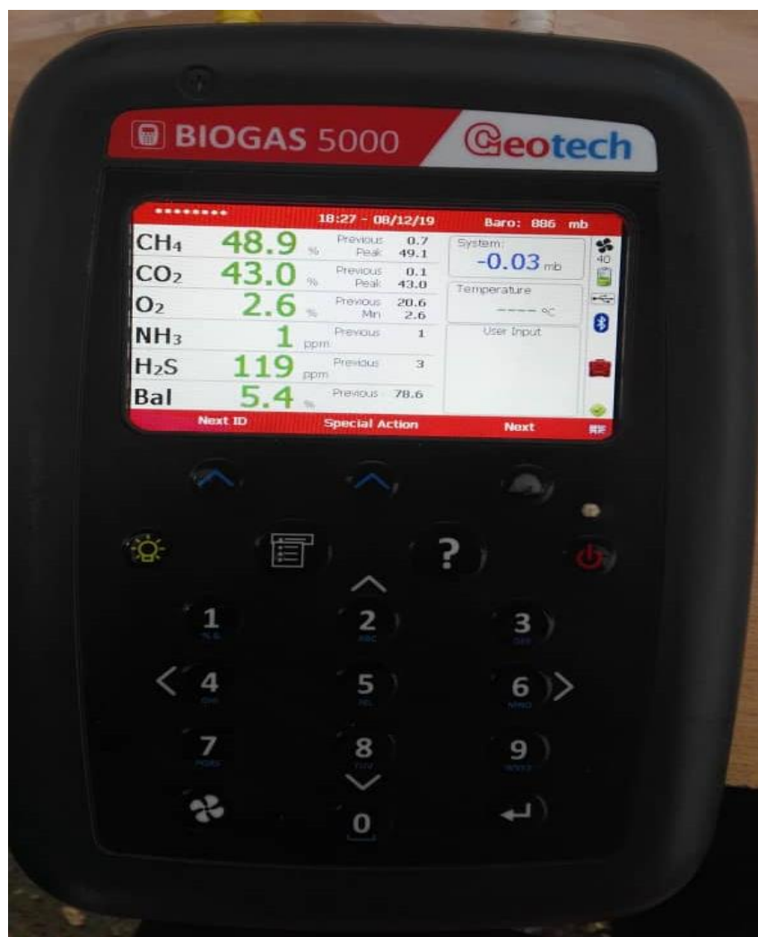
Figure 3: Geotech Biogas 5000 analyzer
