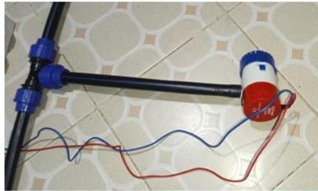
Water Pump and T-Junction pipe
