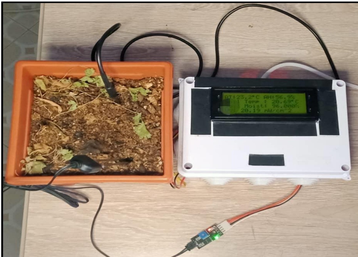
Figure 45: Wireless sensor node calibration set-up
