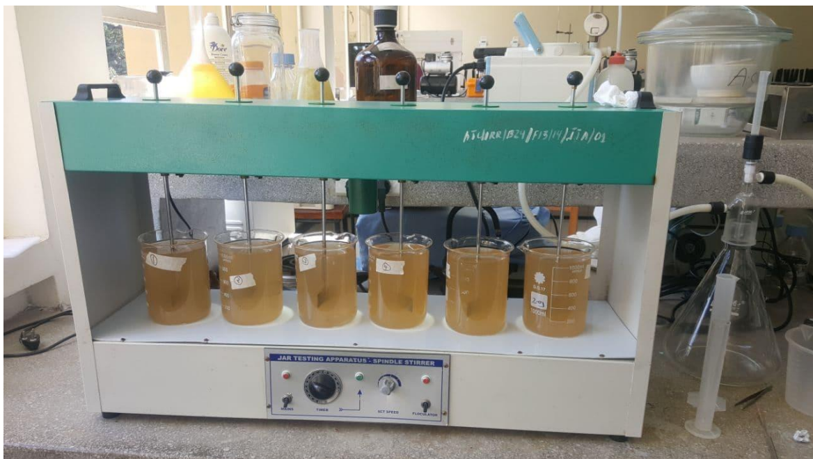
Figure 2: A laboratory set up of the jar-test apparatus
