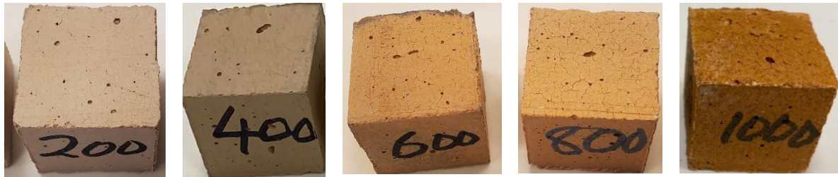
Figure 24: Images of geopolymer specimens after exposure to elevated temperatures
