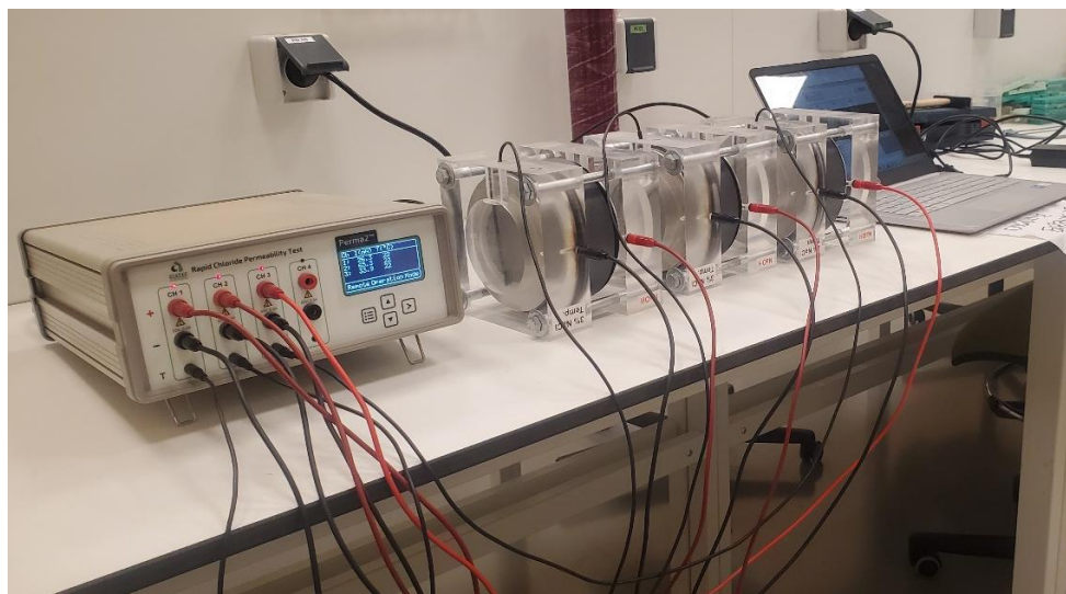
Figure 7: Rapid Chloride Permeability Test Setup
