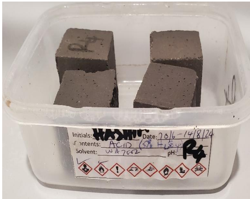
Figure 6: Sulphuric acid immersion of geopolymer mortar specimens
