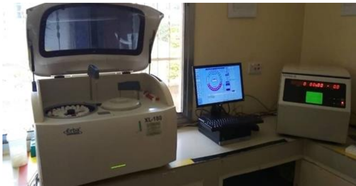
Figure 5: CRP analysis using ERBA (Mannheim) automated clinical chemistry analyser XL 180
