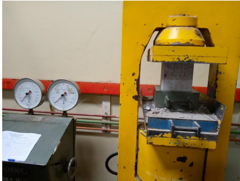
Figure 10: Compressive strength testing machine
