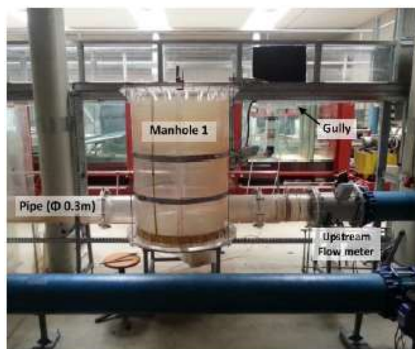
Figure 8: Manhole experiment at Coimbra laboratory
