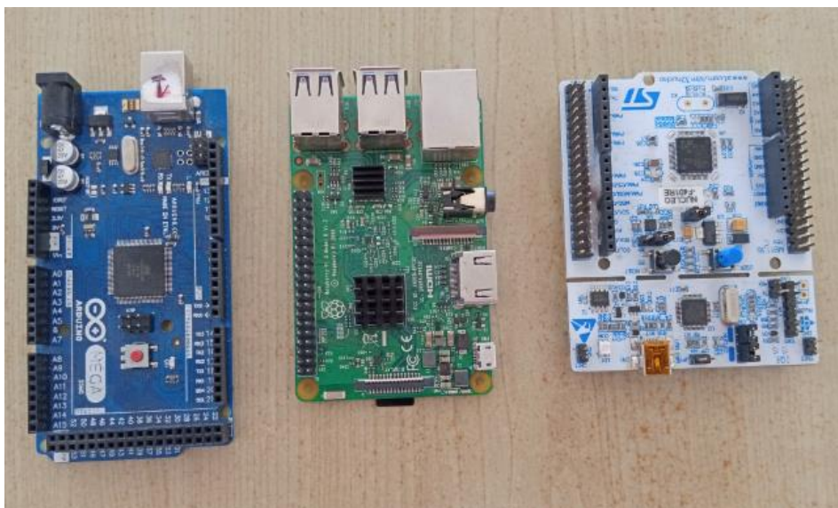
Figure 18: Atmega2560, Raspberry Pi and Nucleo-F410re microcontroller boards
