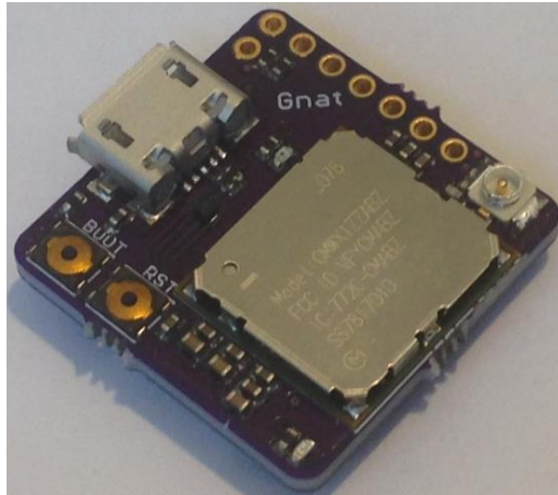
Figure 19: LoRa module used for data transmission (Hackaday, 2018)
