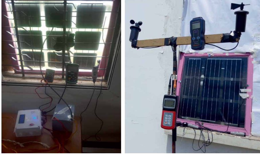
FIGURE 2: The inside and outside view of semi-transparent PV glazing on the window.
