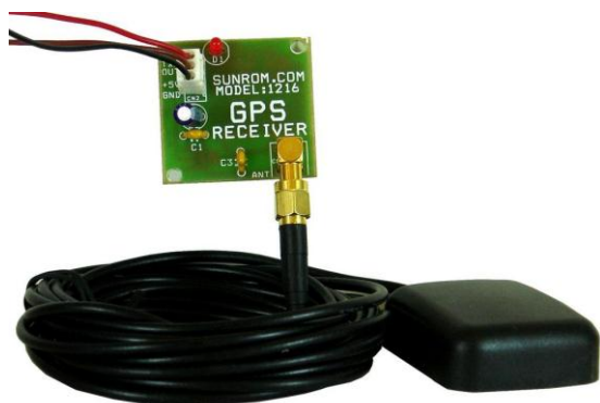
Figure.3: GPS Receiver with Active Antenna
