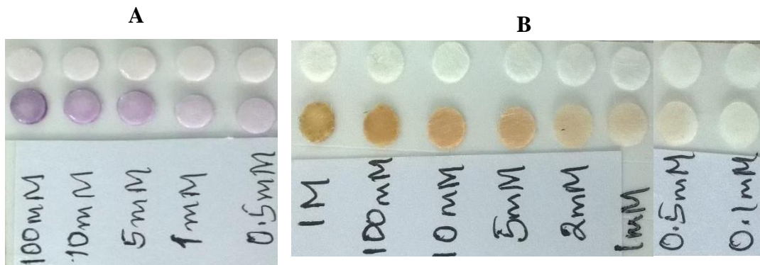
Figure 16. Test discs for Uric acid and Glucose tests.
