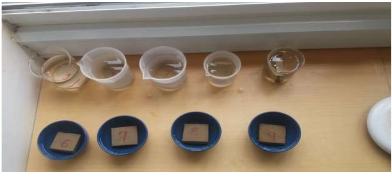
Figure 5: Determination of bulk density, water absorption and porosity using Archimedes principle
