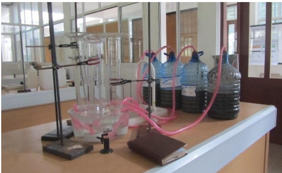
Figure 4: Experimental laboratory set up for biogas production basing on different mixing ratios
