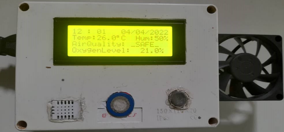
Figure 26: System displaying oxygen, air quality and temperature levels in safe mode
