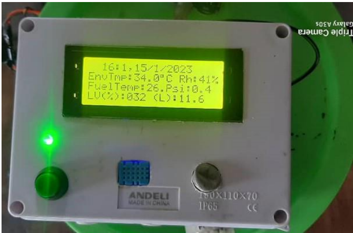
Fig. 23. Final Developed Prototype for Fuel Monitoring System.
