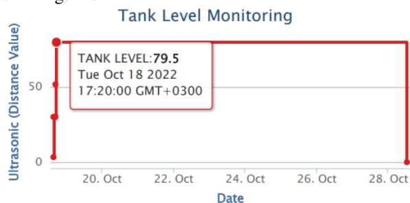
Fig. 12. Visualization of ultrasonic sensed fuel level values.
