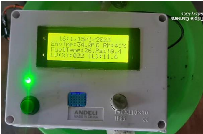
Fig. 23. Final Developed Prototype for Fuel Monitoring System.
