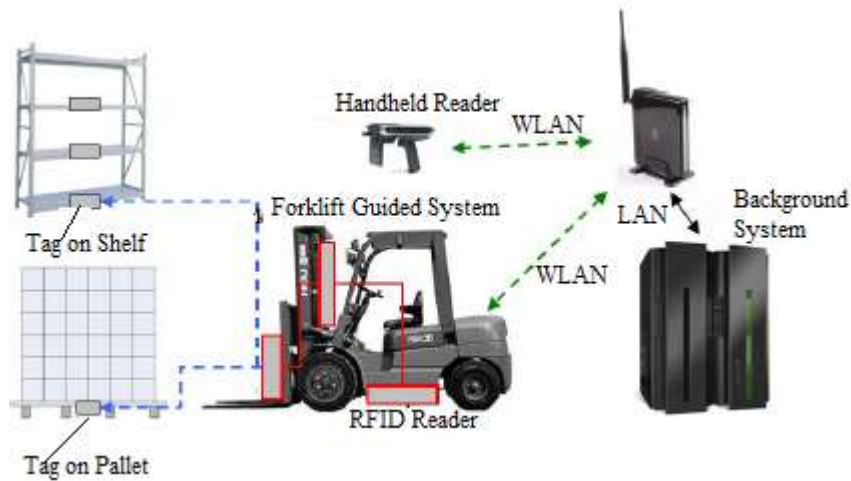
Figure 4. Functionality of RFID based forklift guides system
