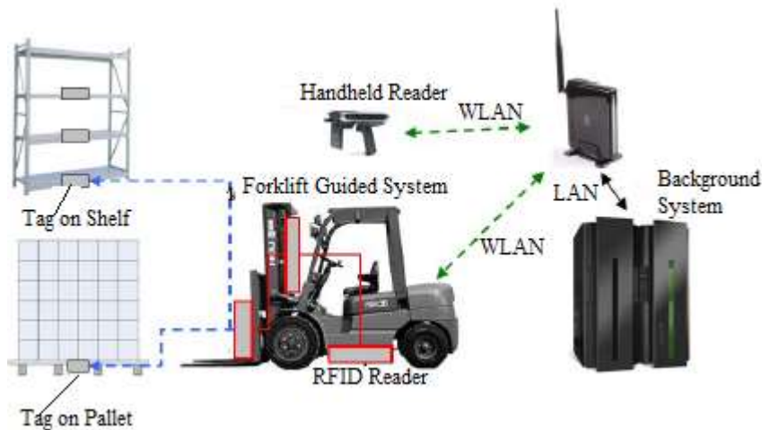
Figure 4. Functionality of RFID based forklift guides system
