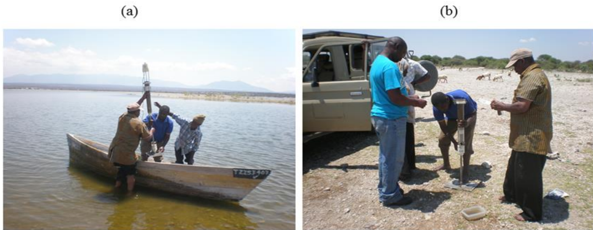
Plate (1): Sampling of sediment core from Nyumba ya Mungu Reservoir, (a) local boat was used to sample at the centre of the reservoir with core sampler, (b) sediment slice of 1 cm thickness was cut and each kept in plastic bag.
