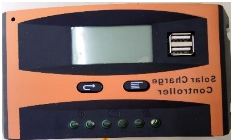
Figure 6: Solar charge controllers
