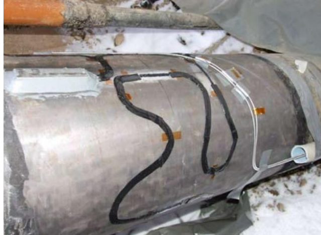
Figure 5: Optical fiber fuel monitoring system attached with optic fiber sensors
