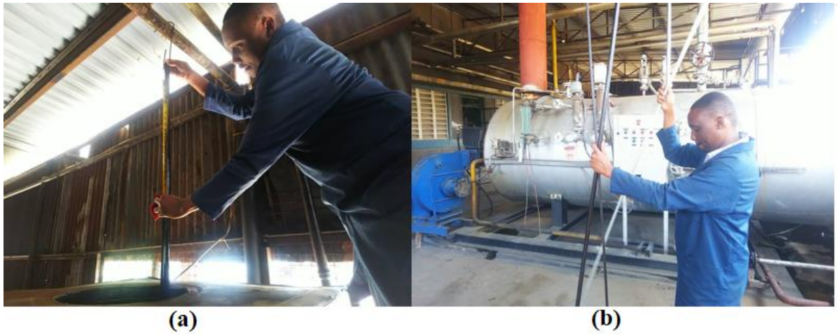
Figure 11: Fuel monitoring (a) using stick and tape measure in fuel tank (b) Graduated stick in storage tank
