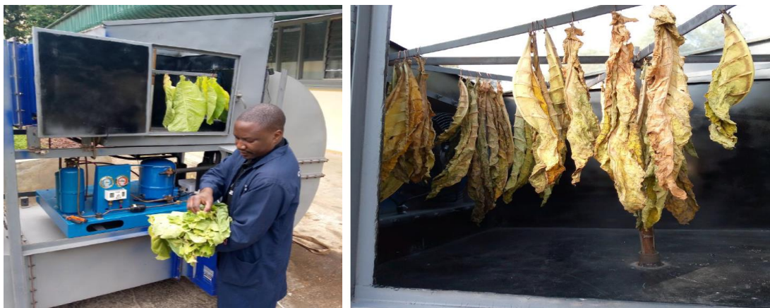
Figure 5: Drying tobacco leaf inside the drying chamber
