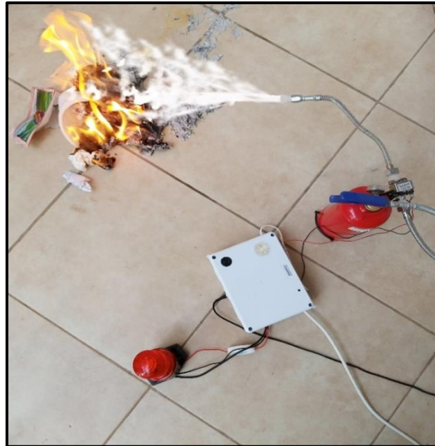
Figure 25: Detection of fire with real-time extinguishing
