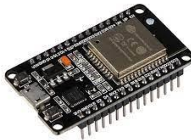
Figure 3: ESP WROOM 32 (Islam et al. , 2020)
