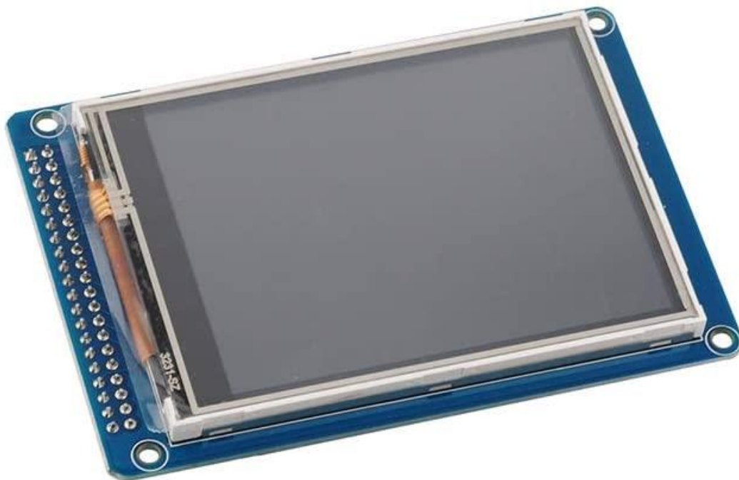
Figure 8: LCD display (Mohamad et al. , 2020)
