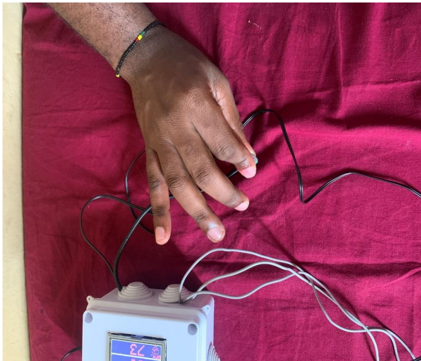
Figure 21: Heart rate and Spo2 measurement
