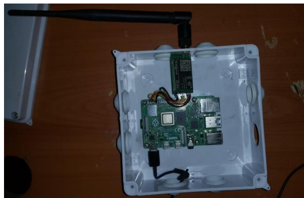
Figure 16: Internal view of the coordinator
