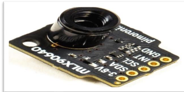
Figure 4: MLX90640 far-infrared thermal camera
