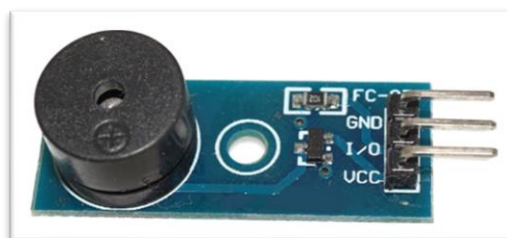
Figure 7: Alarm module buzzer (Devices, 2019)
