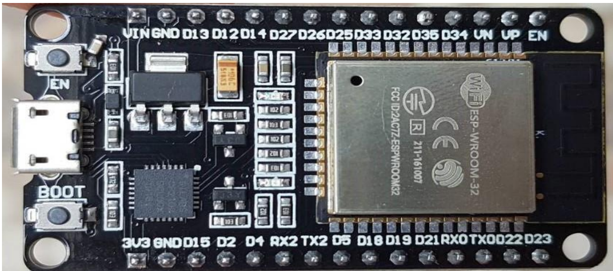
Figure 7: Espressif Systems 32 microcontroller board (Randomnerdtutorials, 2013)
