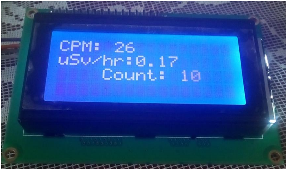
Figure 23: Radiation data visualization on Liquid Crystal Display
