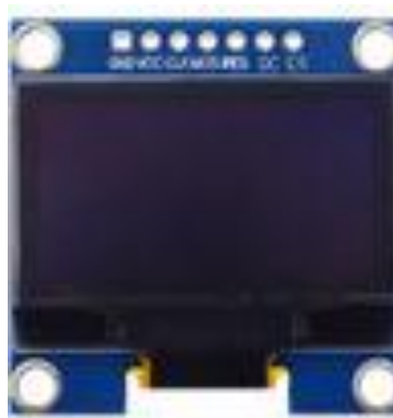
Figure 5: Organic Light Emitting Diode
