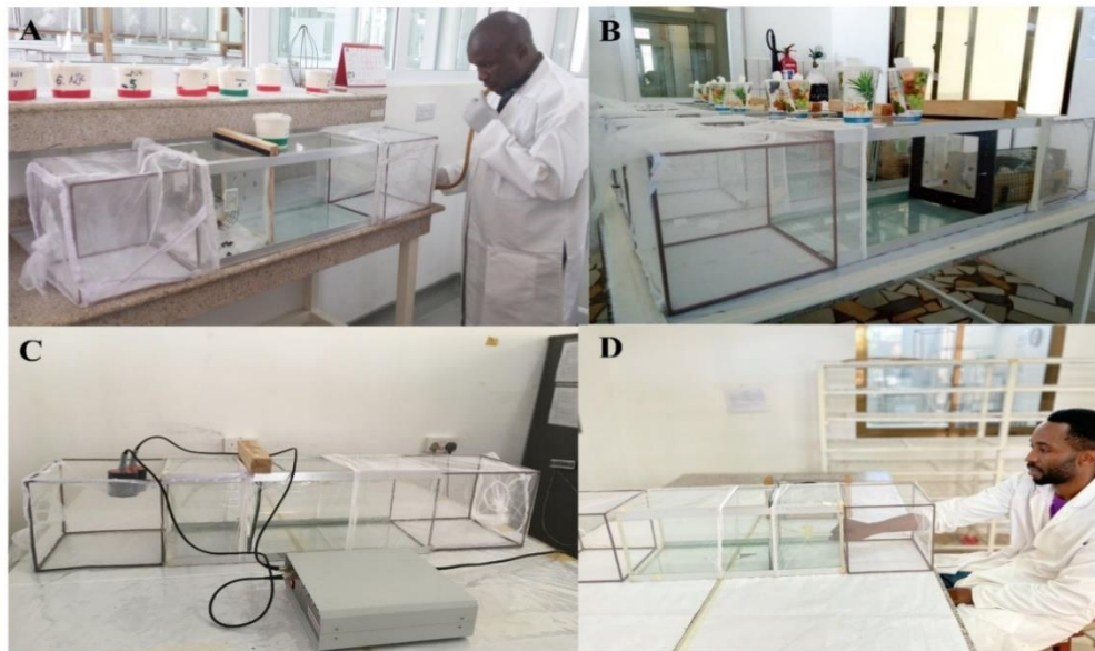
Figure 1: WHO tunnels for comparison of baits/hosts
