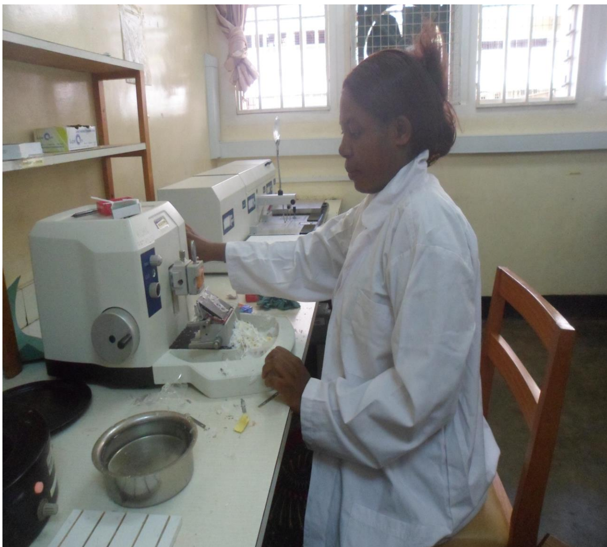
Figure 5: Microtome machine used for slicing tissue biopsies
