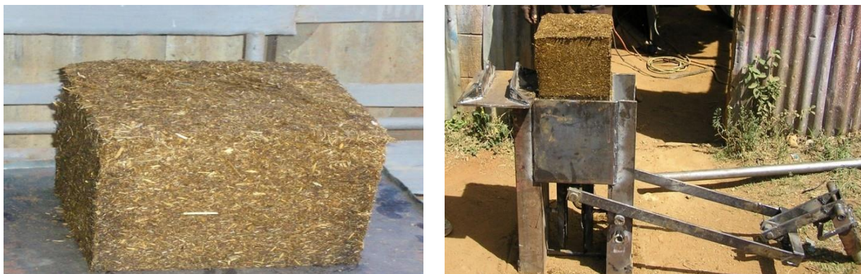
Figure 6: Urea and Urea plus molasses pre-treated maize stover compacted into 5 kg feed blocks using a local feed compactor
