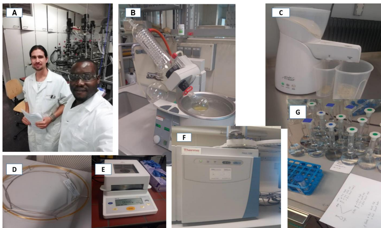
Plate 2: Laboratory analyses showing “A” researcher during analyses, “B” Petroleum ether recovery during the analysis of fat, “C” oyster nut oil cold extraction using Soxhlet extractor, “D” gas chromatography column used for methyl esters separation, “E” rapid moisture analyzer, “F” gas chromatograph used for methyl esters analysis, “G” 10 mL volumetric flasks during mineral analyses
