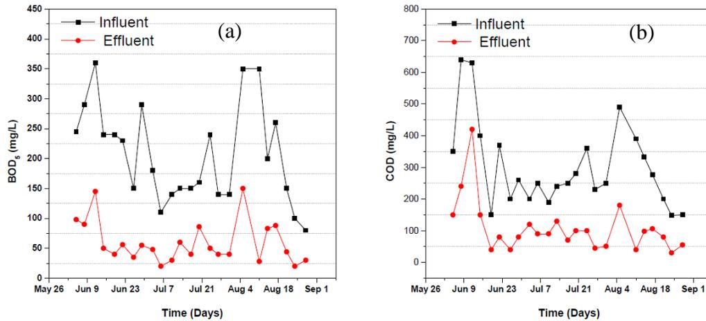
**Figure 15: The variation of (a) BOD<sub>5</sub> (b) COD pollutants with time in HSSFCW at the influent and effluent**
