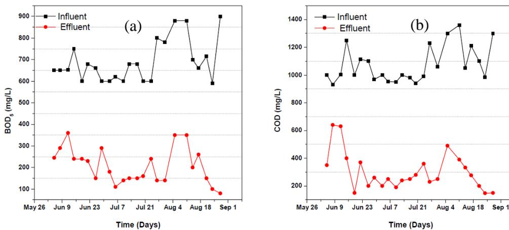
**Figure 10: The variation of pollutants with time in ABR at the influent and effluent (a) BOD<sub>5</sub> (b) COD**
