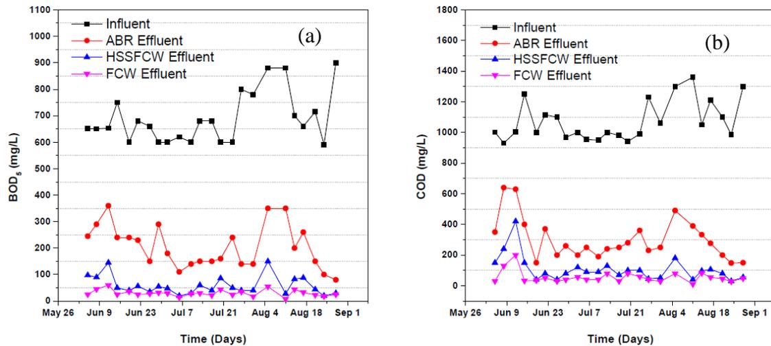
**Figure 24: Pollutant concentration variation in each treatment unit with time (a) BOD<sub>5</sub> (b) COD**
