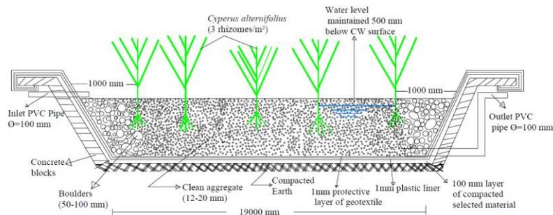
**Figure 5: The cross-sectional area of HSSFCW unit**
