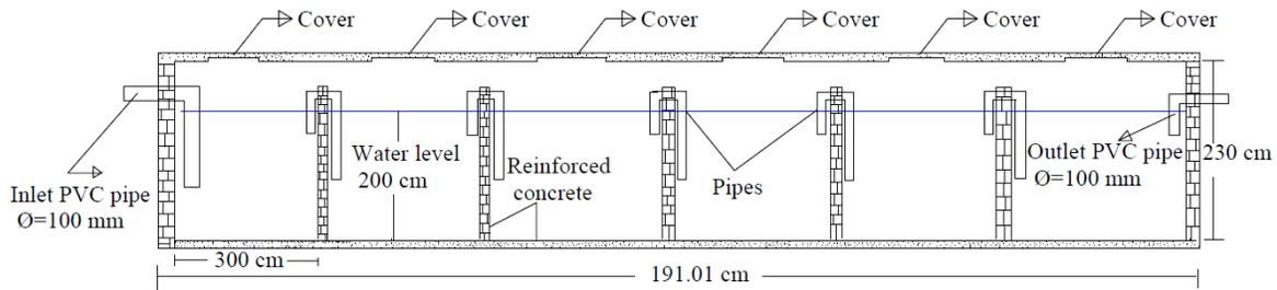
**Figure 4: The cross-sectional area of ABR unit**
