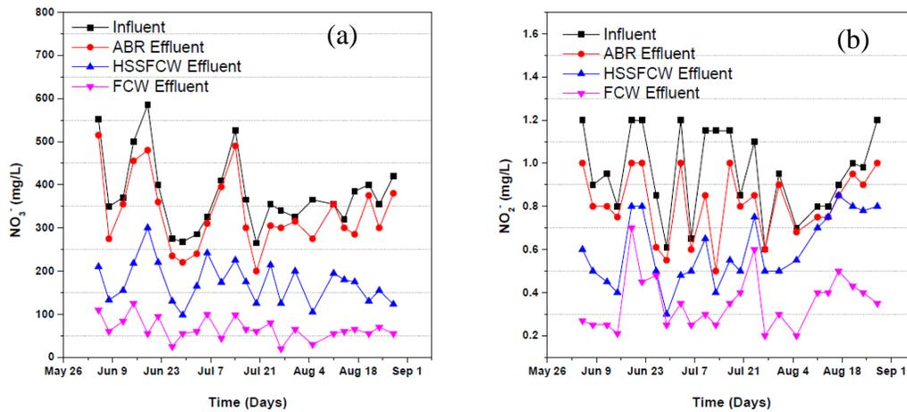
**Figure 25: Pollutant concentration variation in each treatment unit with time (a) NO<sub>3</sub><sup>-</sup> (b) NO<sub>2</sub><sup>-</sup>**
