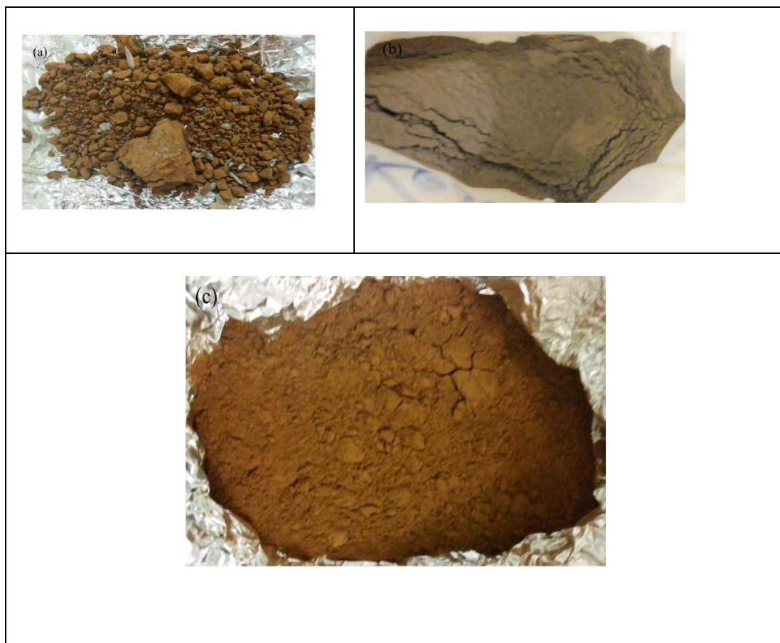
Figure 4: Adsorbent samples from (a) red rock soil (b) Fine powder of anthill soil (c) Fine powder of red rock soil
