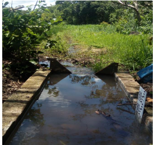
Figure 3: Field measurement of irrigation water using V-notch
