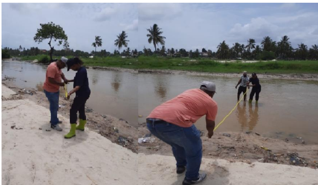
Figure 8: Msimbazi river depth measurement process
