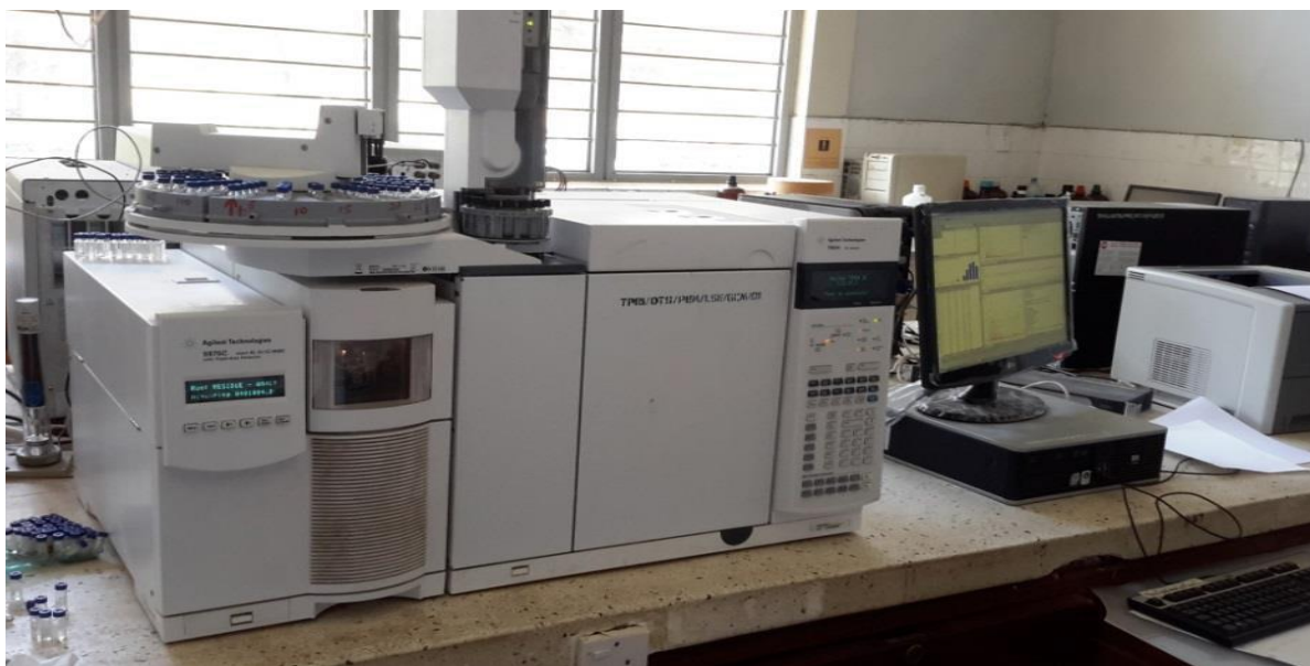
Figure 3: A Gas Chromatography connected to the Mass Spectrometer instrument used in the study
