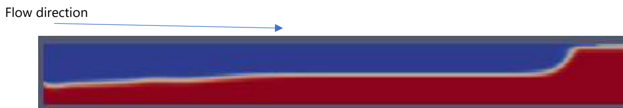
Figure 5: Liquid and Air Flows inside a Pipe for 1.0m Diameter at 3 degrees
