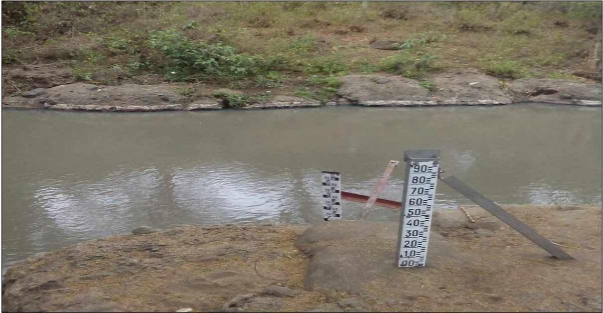
Figure 1: Stage boards for monitoring river water level
