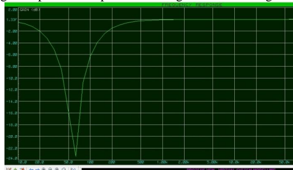
Fig. 5 Notch Filter Frequency Response
