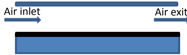
Figure 1. Schematic view of single duct solar collector.
