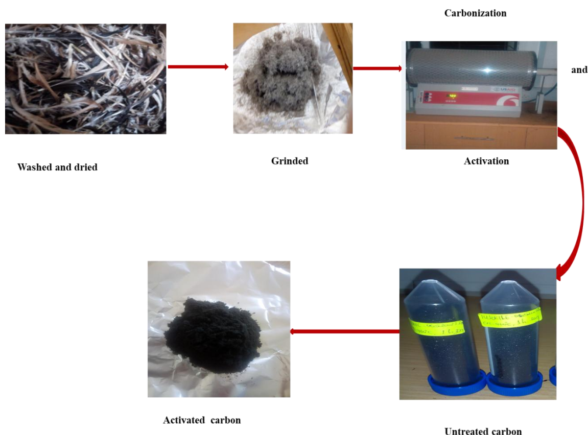
Figure 2: Schematic illustration of the synthesis of chicken feather derived carbon.
