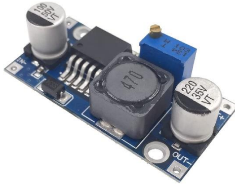
Figure 26: The LM2596 step down module
