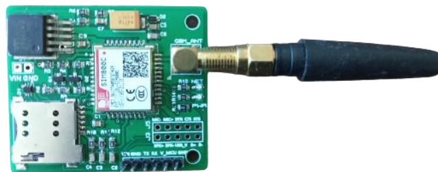
Figure 24: The GSM SIM800C module
