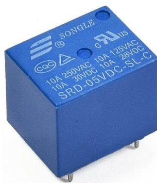
Figure 30: The SRD-05VDC-SL-C relay
