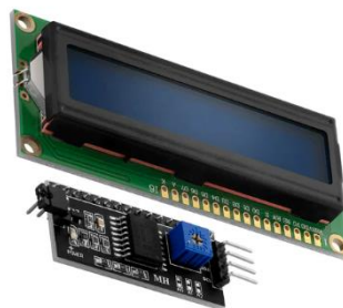
Figure 20: The 16 x 2 LCD display and I2C interface adapter
