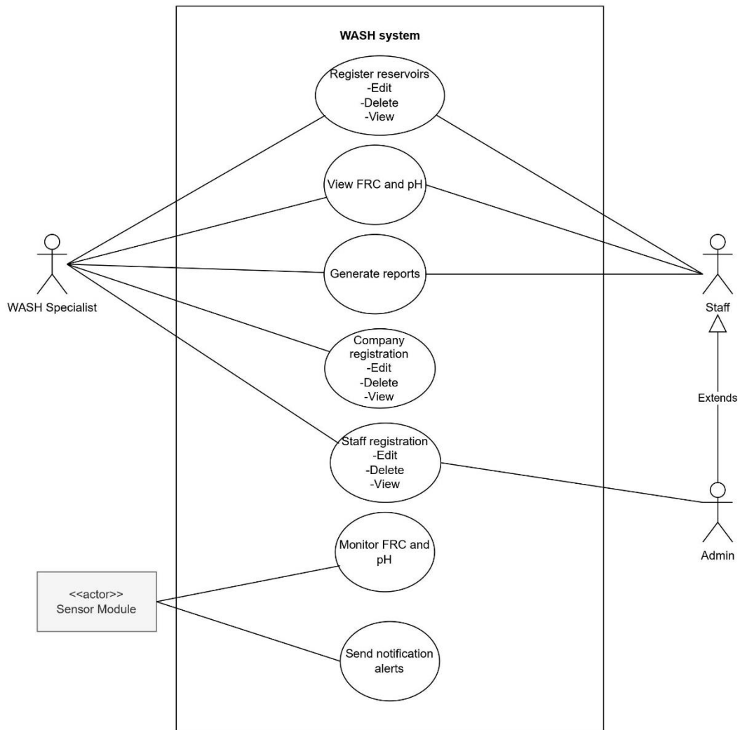
Figure 12: Use case diagram of the system
