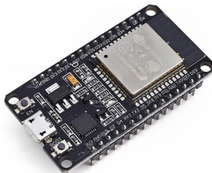
Figure 19: The ESP32-WROOM-32 development board
