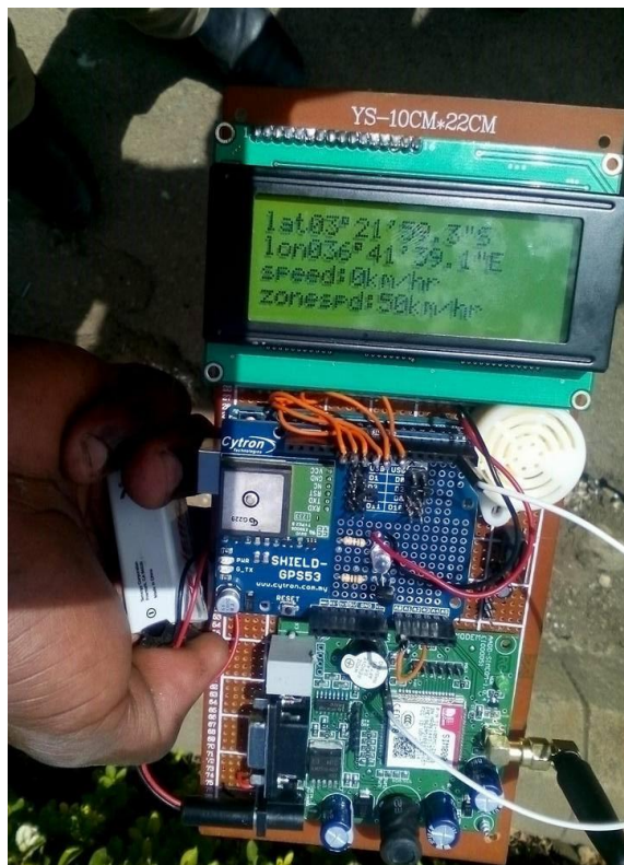
Figure 9: Snapshot of a system in action detecting a speed zone and display location and vehicle speed
