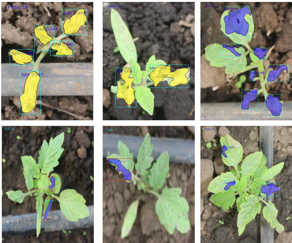
Figure 41: Examples of quantification results carried out by the OpenCV function built on top of the proposed Mask RCNN model
