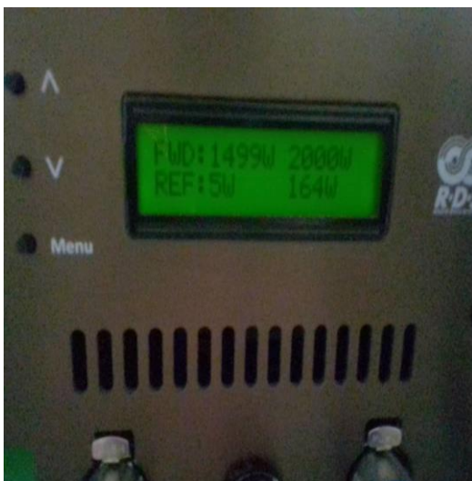
Figure 39: Appearance of the real transmitter's display and its correspondence prototype transmitter
