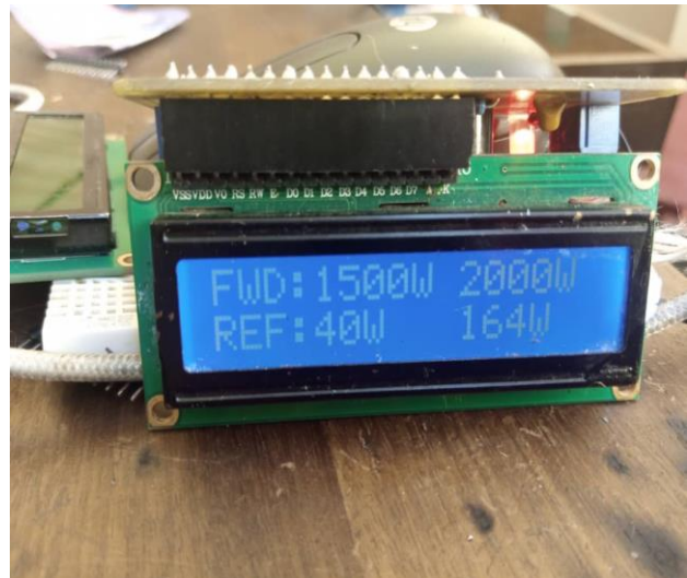
Figure 39: Appearance of the real transmitter's display and its correspondence prototype transmitter
