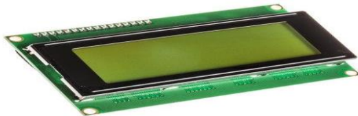
Figure 8: The LCD 20x4 Display
